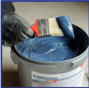
**Liquid Brush—Blue** Available in 5Kg and 2.5Kg tubs this is the most widely used form of Blowerproof. The fibre reinforced polymer has a viscous consistency not unlike mayonnaise, and simply brushes on. Two coats are normally recommended, apply the second when the first coat has turned from blue to black. Maximum thickness per layer 5-7mm maximum total thickness 10-14mm. Apply to any dust free stable surface. Gaps wider than 5mm should be filled with Blowerproof gap Filling Mortar.
