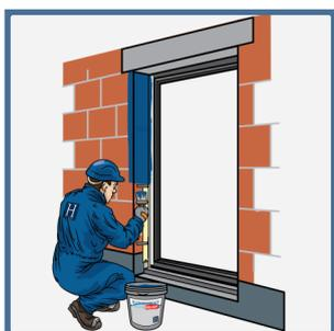
**Window jambs** are so simple and quick to seal, first fill larger gaps between the window frame and the wall with PU foam, then apply protection tape on the profiles at about 5mm from the side, next simply brush on Blowerproof Liquid Brush directly onto the wall and window surfaces (and over the hardened gap filling foam) remove the tape immediately after application, any spills can be easily cleaned with water.
